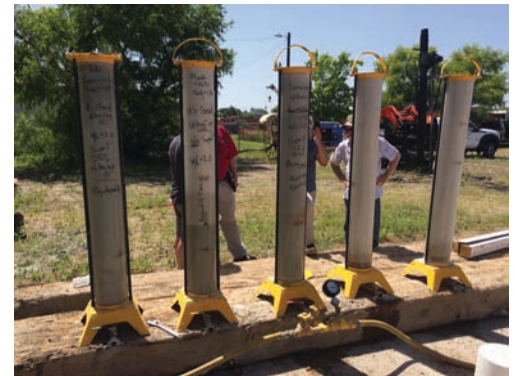
Field Demo: Sand column grouting tests with different types of Microfine cement.
