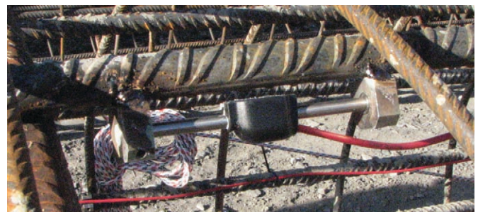
Figure 1b. Strain gage embedded in concrete.
