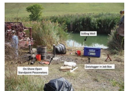
Figure 5. On-shore monitoring location and on-shore open standpipe piezometers.
