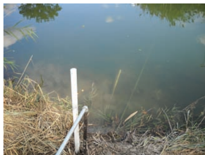
Figure 4. Stilling well and pipe protection of cables.
