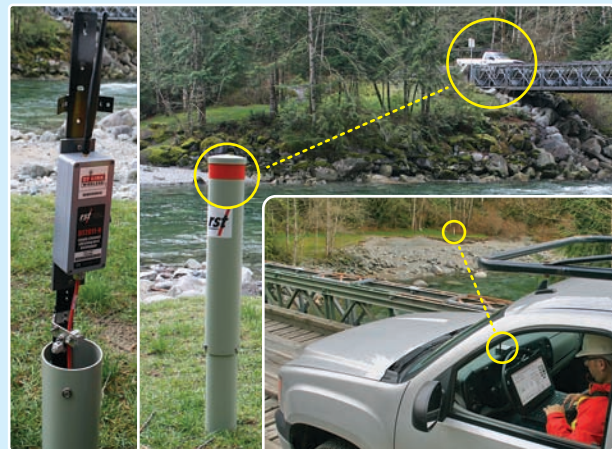
Above: A DT LINK WIRELESS data logger, connected to a vibrating wire piezometer and housed in a protective enclosure, has its data collected from a laptop connected to the DT LINK HUB - all within seconds from the convenience of your vehicle.
