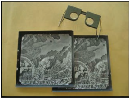
Figure 2. Hardcopy aerial photographs and stereoscope.
