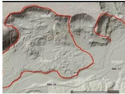
Figure 3. LiDAR data showing area of past landsliding
