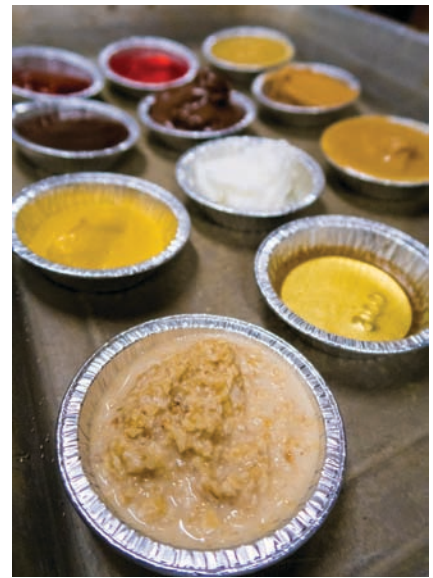
Figure 4. Geotechnical moisture test samples ready for the oven.
