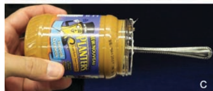
Figure 5. Spoon test: A - condensed milk (0.07 kPa fail); B - ketchup (0.22 kPa pass vertical); C - peanut butter (1.8 kPa pass horizontal). Spoon will stand vertical if >0.2 kPa, horizontal if >0.4 to 0.8 kPa.
