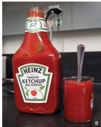
Figure 6. Pour test. A - fluid fine tailings (0.07kPa); B - chocolate milk (0.05 kPa); C - yogurt (0.4 kPa). Materials pour if <0.3 kPa.
