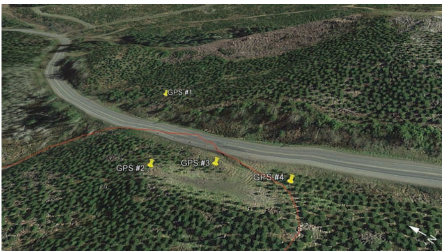
Figure 4. Layout of GNSS receivers on site (red line shows the outline of the landslide).
