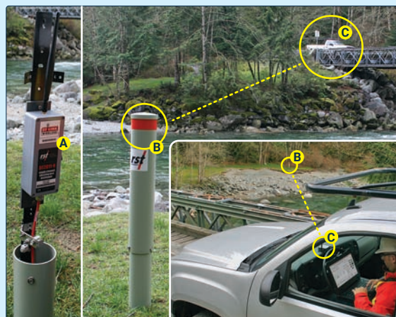
Pictured: (A) DT LINK WIRELESS data logger, connected to a vibrating wire piezometer and housed in a (B) protective enclosure, has its data collected from a laptop connected to the (C) DT LINK HUB - all within seconds from the convenience of your vehicle.
