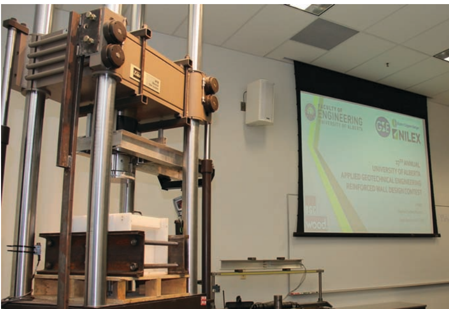
Instrumented loading frame used to test the reinforced soil walls.
