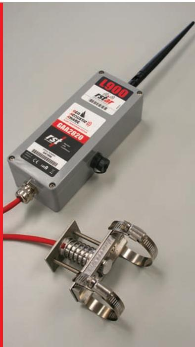
The Geo-Acoustic Aware (GAA) Slope Monitoring System from RST is a **low-cost, reliable solution** for the spatial infill of ground movement data at shallow depths. It provides **early warning of movement** when monitoring slow to moderate slope movement rates in:
