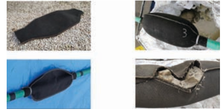
Figure 10: Folded and injected obturator bags mounted astride a manchette.
