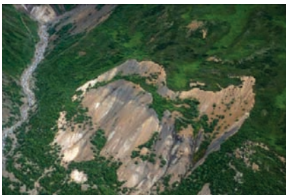
Figure 5a: Geohazards affected by seismic and precipitation triggers, landslide triggered by seismic activity on the Denali Fault, Alaska (photo ©Rod Read, used by permission).
