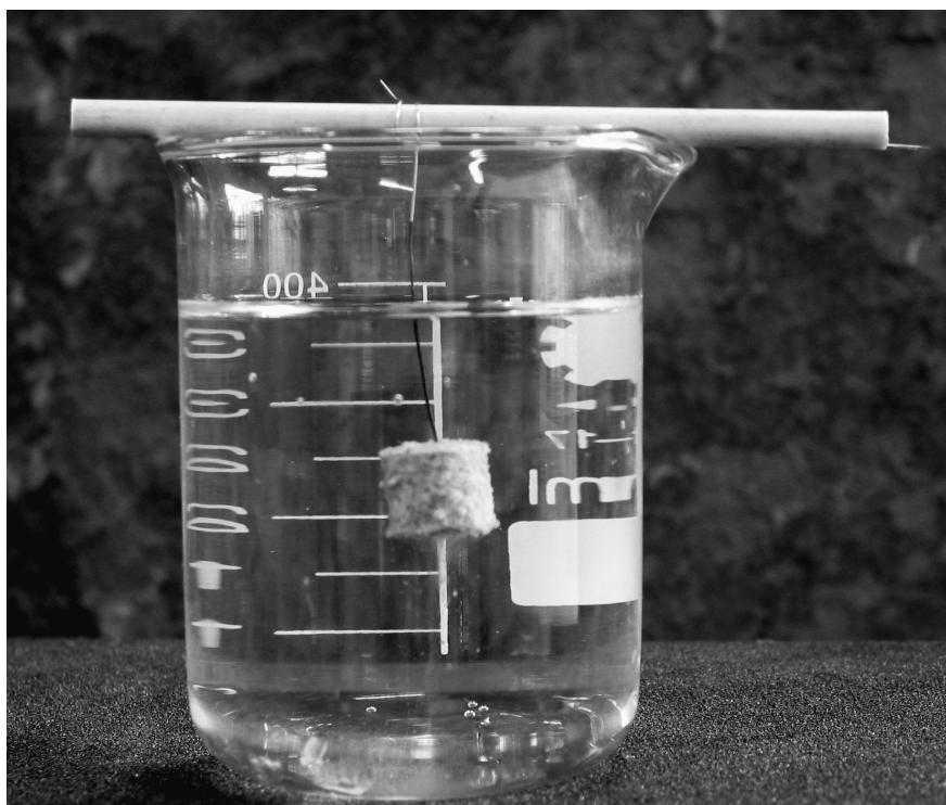
Figure 5. 400mL beaker used to determine the time to stickiness of bentonite. Stickiness was measured by recording the time at which the sample was able to stick to the side of the beaker.
