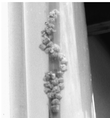
Figure 3. Onset of bridging with 1/4" uncoated pellets.
