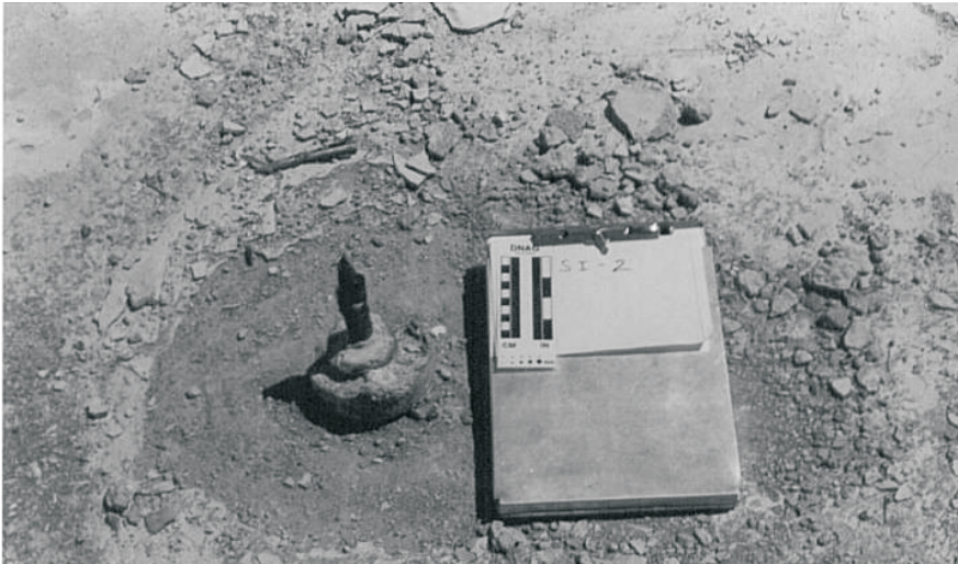
Figure 5. Installation of TDR sensor cable in sheared inclinometer casing extends the life of the monitoring borehole
