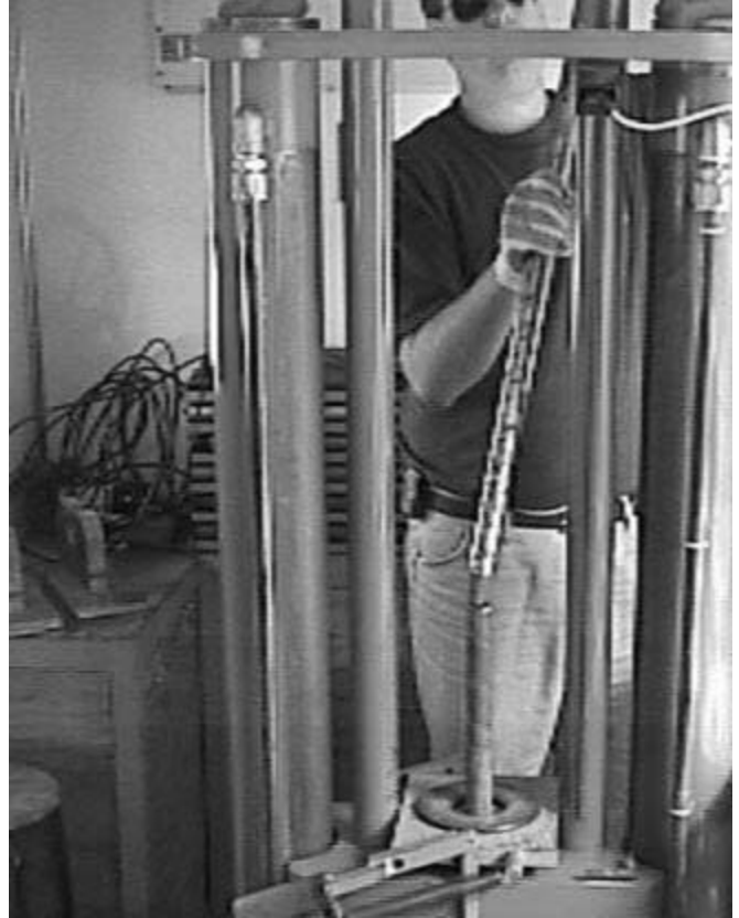
Figure 9. Insertion of TDR sensor cable in CPT rods after attaching special disposable tip
