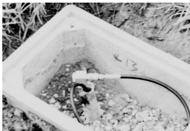
Figure 12. Protective enclosure for connection between a sensor and a connecting cable
