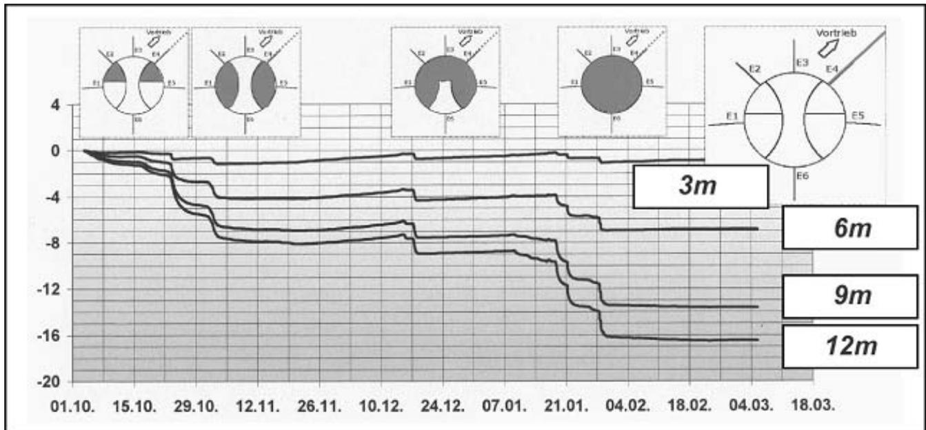
Figure 13. Displacements recorded over time in the Uetlibergtunnel in Switzerland during different excavation stages
