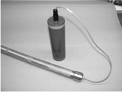
Figure 12. Multipoint extensometer head with radio transmission module
