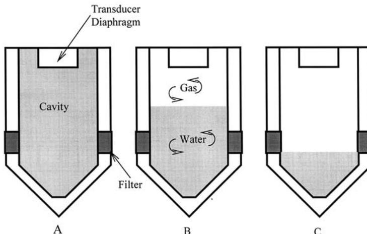
Figure 1. Effect of gas production on conditions within a piezometer cavity
