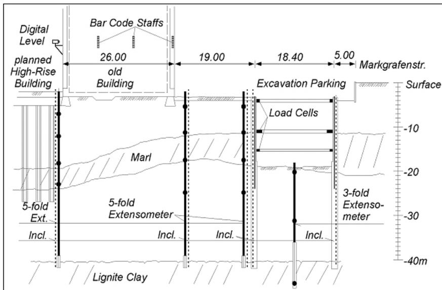
Figure 8. GSW-building Berlin. Cross section, geology, constructional measures, instrumentation
