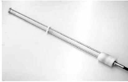
Figure 4. Dual rod TDR probe
