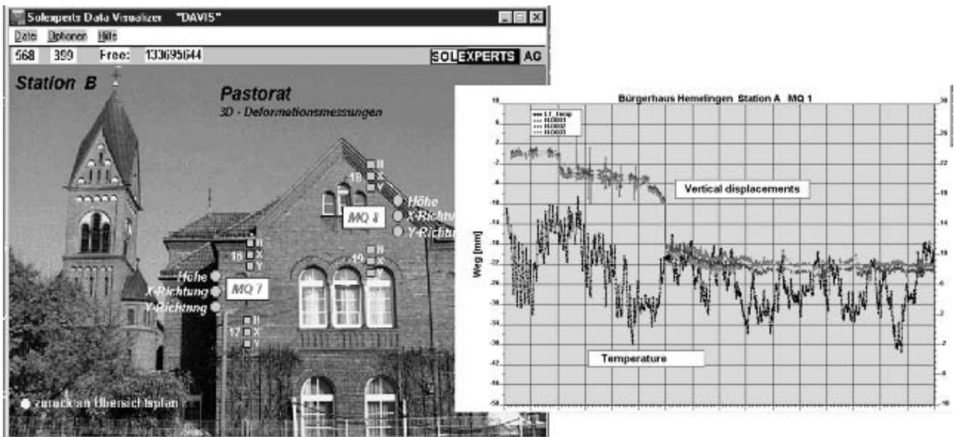
Figure 11. Building with the measuring points installed at a tunnelling project in Bremen, and a graph with settlement and air temperature versus time.
