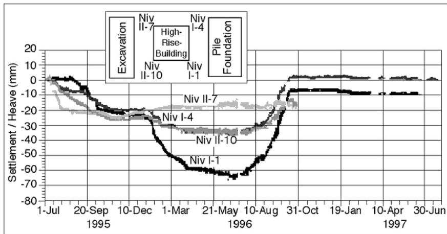
Figure 9. Settlement and heave due to construction
