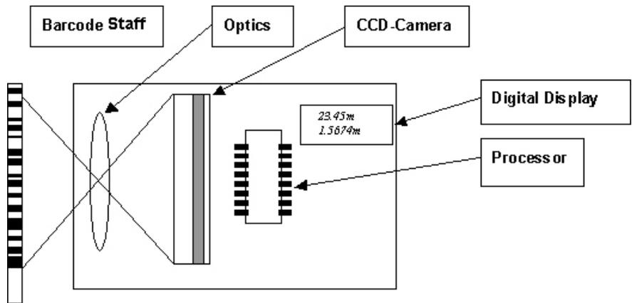
Figure 6. Schematic layout of a digital level
