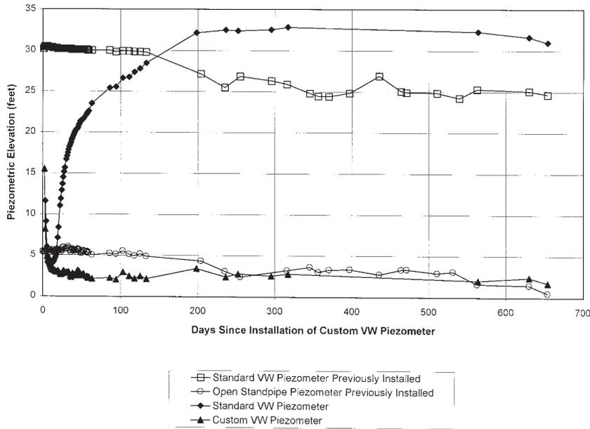
Figure 4. Piezometric elevations at Instrument Cluster 2
