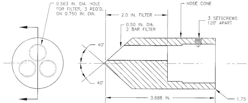
Figure 2. Detail of custom-designed VW high air entry piezometer
