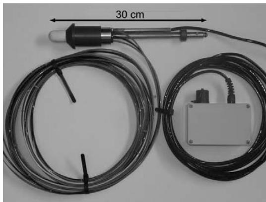
Figure 2. A new flushable piezometer with removable sensor
