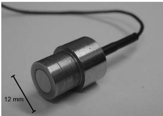
Figure 1. A suction probe for measuring pore pressures below minus one atmosphere
