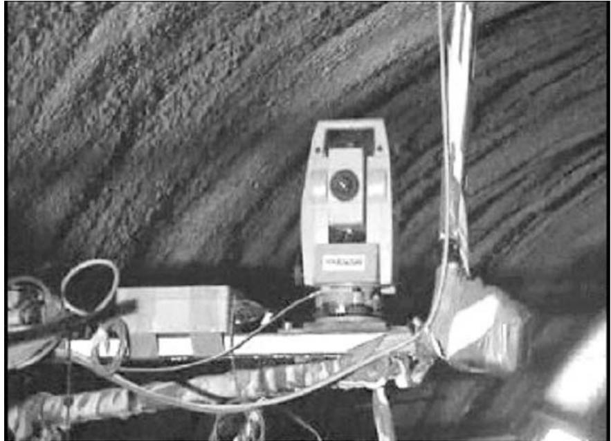
Figure 10. Total station for monitoring the Zurich Zimmerbergtunnel
