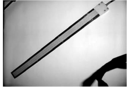
Figure 5. TDR probe for monitoring water content in the interface between a bentonite seal and concrete
