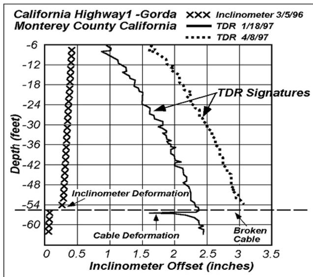
Figure 3. TDR-signatures and inclinometer reading during landslide monitoring
