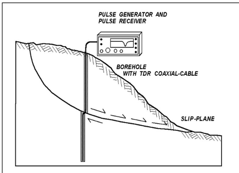
Figure 2. Schematic of TDR instrumentation for landslide monitoring
