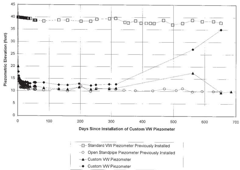
Figure 3. Piezometric elevations at Instrument Cluster 1
