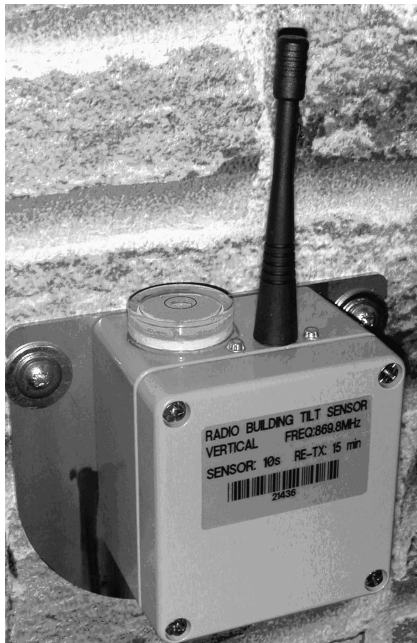
Figure 2. Integrated sensor and transmitter to form a complete cable-free tiltmeter.
