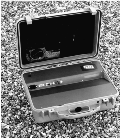
Figure 6. Portable SOFO system readout unit.
