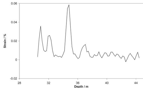
Figure 3. Strain profile measured with BOTDR in a pile after curing, during which one level of basement was excavated. Peaks are due to cracks up to ~0.3 mm width.
