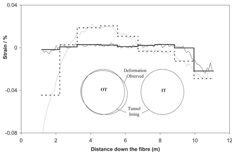
Figure 4. Strain developed around first of twin tunnels during the construction of the second tunnel in close proximity. Solid lines when face of 2<sup>nd</sup> TBM is level with monitoring location, dotted lines when 2<sup>nd</sup> TBM is more than two tunnel diameters past. Thin lines are measured data. Bold lines are strains calculated, knowing attachment points. Inset is a schematic of the movement observed.
