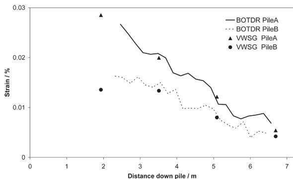
Figure 2. Strain profile measured in a pile group with BOTDR and VWSGs during a static load test at 95% of failure.
