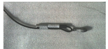
Figure 3. Vibrating wire piezometer with counterweight ready for installation.
