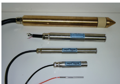
Figure 2. Overview of the piezometers sensors assessed in the laboratory tests. From top to bottom: CL1-750 (A.1), PWF-750 (B.2), PWS350 (B.1), FOP-350 (C), and new MOMS piezometer (D). CL1-350 is identical to CL1-750 and is not shown.
